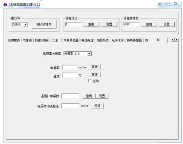
Select the corresponding conductivity resolution according to the purchased equipment range. If you buy a device with a cell constant k=1 with a range of  $1\sim2000 \,\mu$  s/cm, select a resolution of 0.1;
