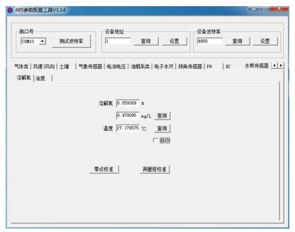
Place the sensor in a 100% oxygen environment. After the dissolved oxygen value is stable, click the full range calibration button to complete the calibration of 100% oxygen saturation.
