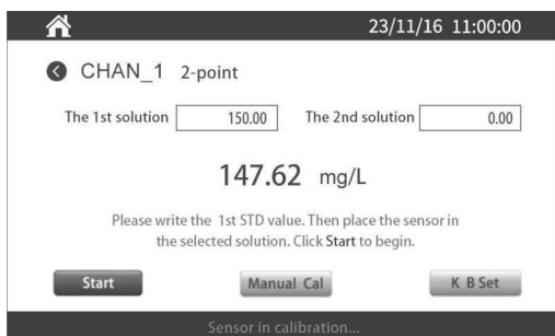
Figure 4.10.3: 1st calibration in progress
