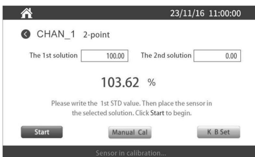
Figure 4.2.3: 1st calibration in progress
