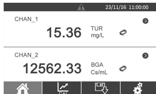
Figure 6.2.4: Main interface alarm
