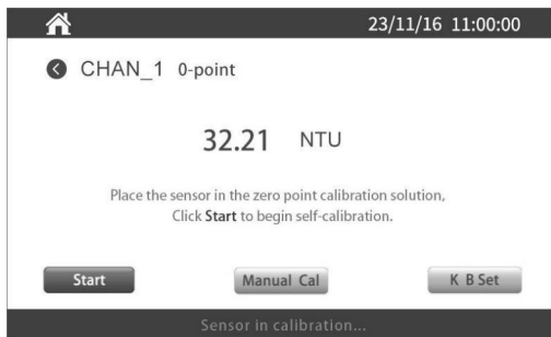
Figure 4.4.1: 0-point calibration in progress
