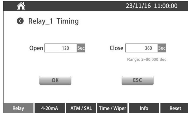
Figure 6.2.2: Relay 1 opens once every 120 seconds for 360 seconds
