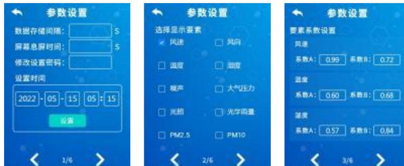
**Data store interval:**Set the device data store interval, the range is 20s~65535s, default is 60s. **Screen off time:**Set the screen off time, the range is 15s~65535s, default is 60s.
