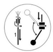
The position of the weight is installed at about 1/2 of the water level to be controlled.
