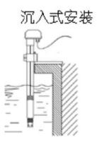
With NPT3/4 thread, it can be used with our waterproof pipe. The cable is inserted from the pipe and the equipment is screwed into the thread of the waterproof pipe.
